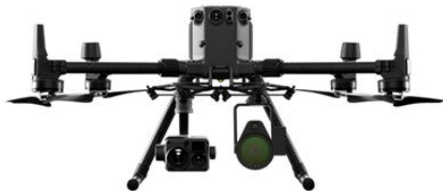
Fig. 2. DJI Matrice 300 RTK drone with Zenmuse H20T payload and U10 gas analyzer
